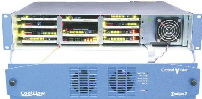
Internal view of Indigo 2SE, which holds up to 12 boards
