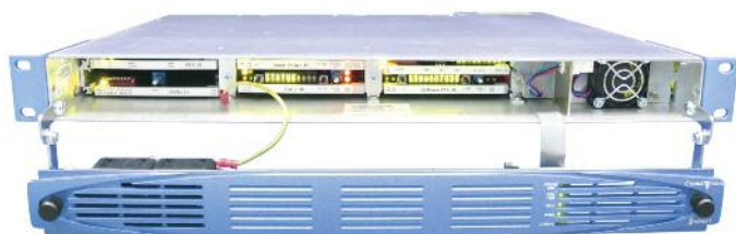
Internal view of Indigo 1SE, which holds up to six boards
