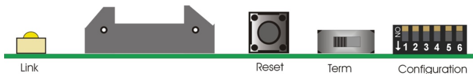
Later model 4U/2U CoolFlow board top-edge switches and LEDs
