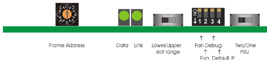
Indigo 2AE board top-edge switches and LEDs
