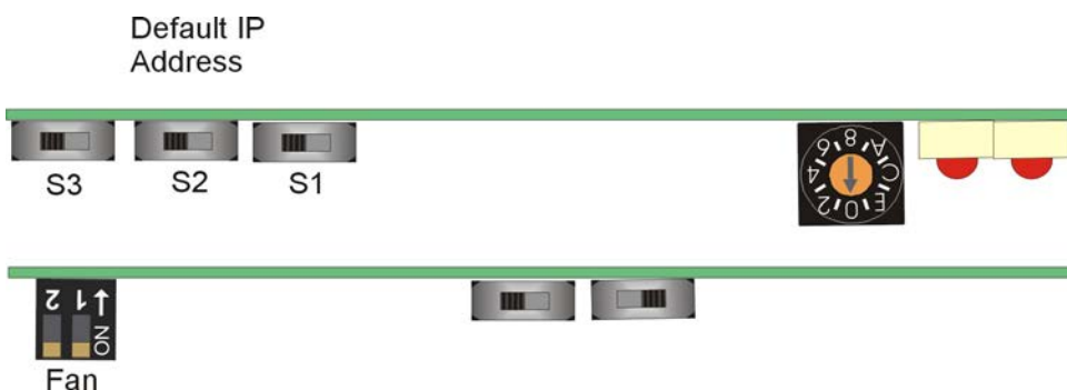
Indigo 1U frame PCB top-edge switches and LEDs
