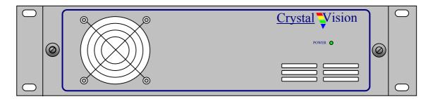
The 2U FR2AV frame will house up to 12 modules and dual power supplies. A hinged front panel gives access to the PSU and all modules. The universal frame wiring system allows any of the interface range of modules to be fitted in any position with the use of removable rear modules.
