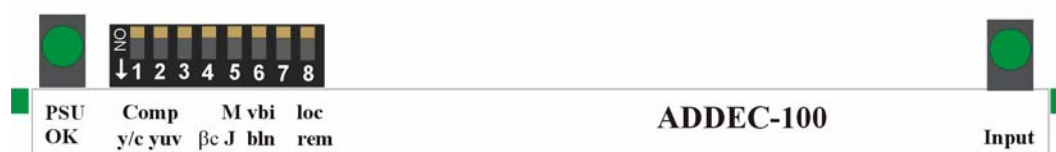
ADDEC-100 front view showing controls and LEDs
