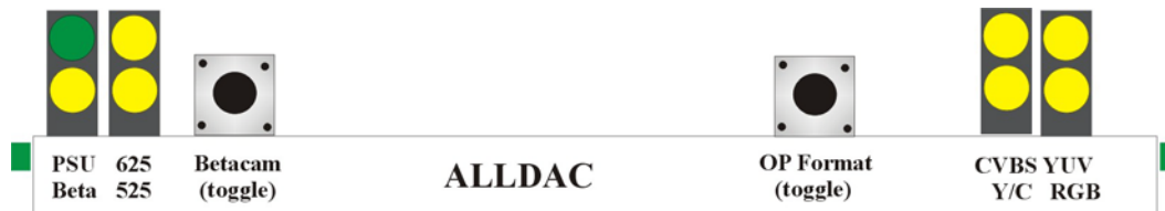
Front view of ALLDAC showing controls and LEDs
