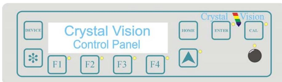
If the control panel firmware has been updated for Statesman control (version 1.5.0 or higher), Statesman Mode will be entered and the message, 'Press CAL to Exit' will be displayed and the CAL LED will light.
