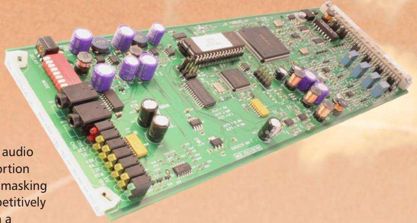
The DACA214 is a dual channel AES/EBU to analogue audio converter. 24 bit processing, excellent noise and distortion figures and Crystal Vision's sophisticated audio error masking together create a truly high quality output. The competitively priced DACA214 offers two independent channels on a 100mm x 266mm module, therefore allowing 24 channels in 2U and making it the perfect audio converter for applications where available rack space is limited.
