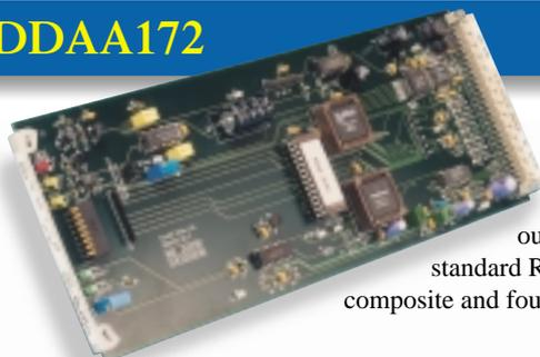
The DDAA172 is an SDI to PAL/NTSC monitoring encoder with distribution amplifier which is ideal where there is a need for many SDI outputs and no requirement for Y/C outputs. It has one input and a maximum of two composite outputs and seven reclocked SDI outputs using a RM02 frame rear module. Using a standard RM01 frame rear module which allows 12 boards in 2U, the DDAA172 offers one composite and four reclocked SDI outputs.
