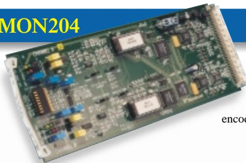
The MON204 is a dual SDI to PAL/NTSC or Y/C monitoring encoder which provides two composite or a single Y/C output for each input. The high-packing density gives 24 encoders in 2U which makes it the obvious encoding choice when SDI loop-throughs are not required.
