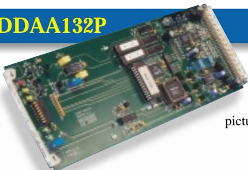
The DDAA132P is identical to the DDAA132 but in addition has four very useful test patterns on the analogue outputs which can be selected by GPI remote control. Patterns include Pluge, which is used to line up picture monitors, and Colour Bars.
