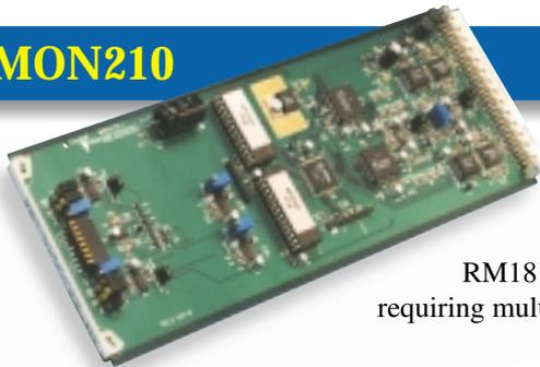
The MON210 is a dual SDI to PAL/NTSC or Y/C monitoring encoder which provides two inputs and a maximum of five composite (or two Y/C pairs and one composite) outputs for each channel when using the RM18 frame rear module. It is the choice for content monitoring applications requiring multiple analogue outputs and no SDI loop-throughs.
