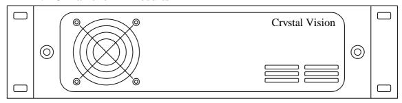
The 2U FR2AV frame will house up to 12 modules and dual power supplies. A hinged front panel gives access to the PSU and all modules. The universal frame wiring system allows any of the interface range of modules to be fitted in any position with the use of removable rear modules.
