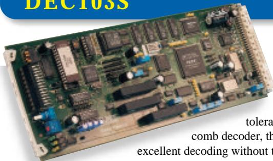
The DEC103S is Crystal Vision's flagship decoder. Aimed at broadcasters, OB facilities and high-end post production, this 10 bit decoder with frame synchroniser is ideal for converting *any* composite or Y/C signals to SDI, and offers very high quality decoding for a fraction of the price of comparable products.
