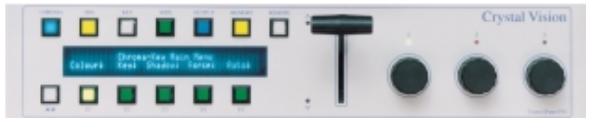
PAN-SKEY remote control panel
