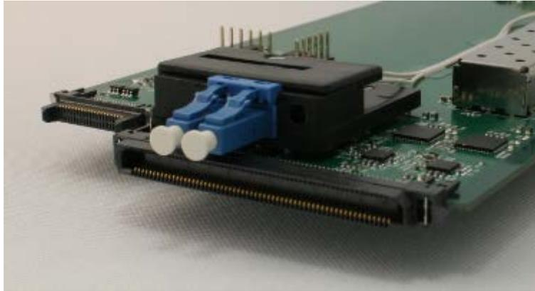
*FRX-VF connectors with the dust caps fitted*
