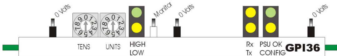
GPI36 front edge view
