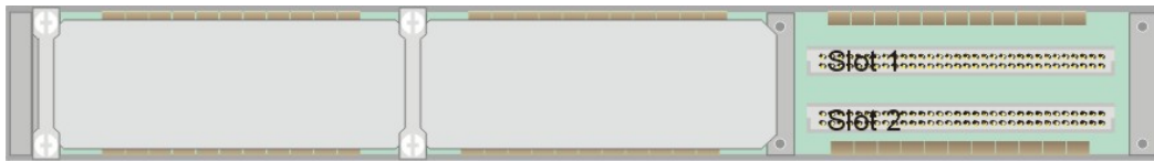
The Indigo 1 frame rear view with EMC covers removed for slots 1 and 2
