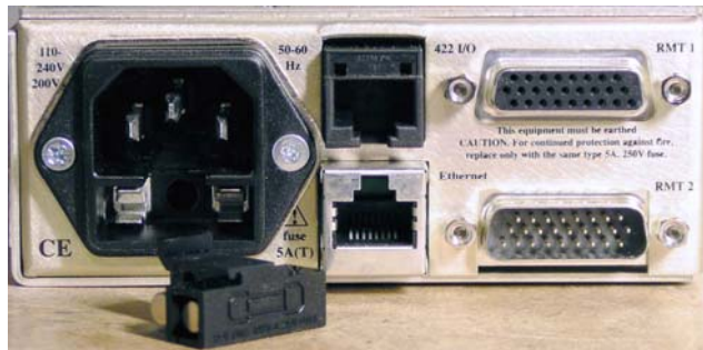
Rear connectors showing IEC mains input and fuse tray with main and spare fuses
