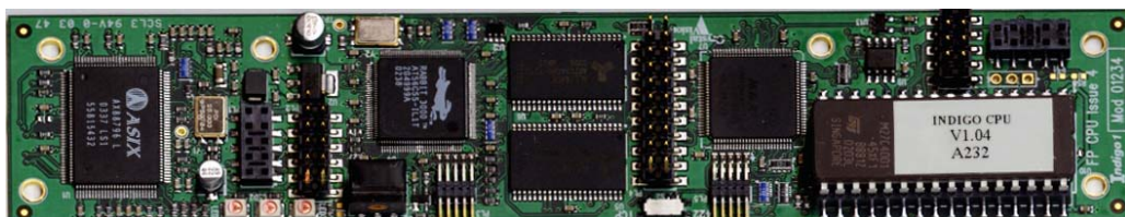
Front panel top PCB showing firmware EPROM in the bottom right corner
