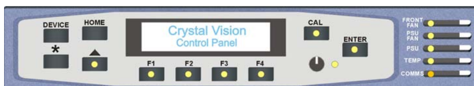
Indigo 1AE active panel controls and LEDs
