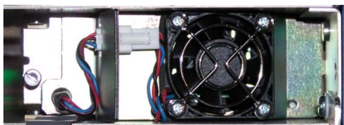
PSU fan showing 3-pin connector and finger guard
