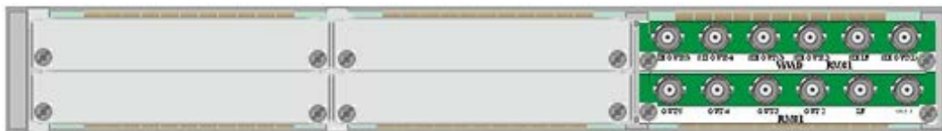
The Indigo 1SE frame rear view with EMC covers fitted and RM01 connectors fitted to slots 1 and 2
