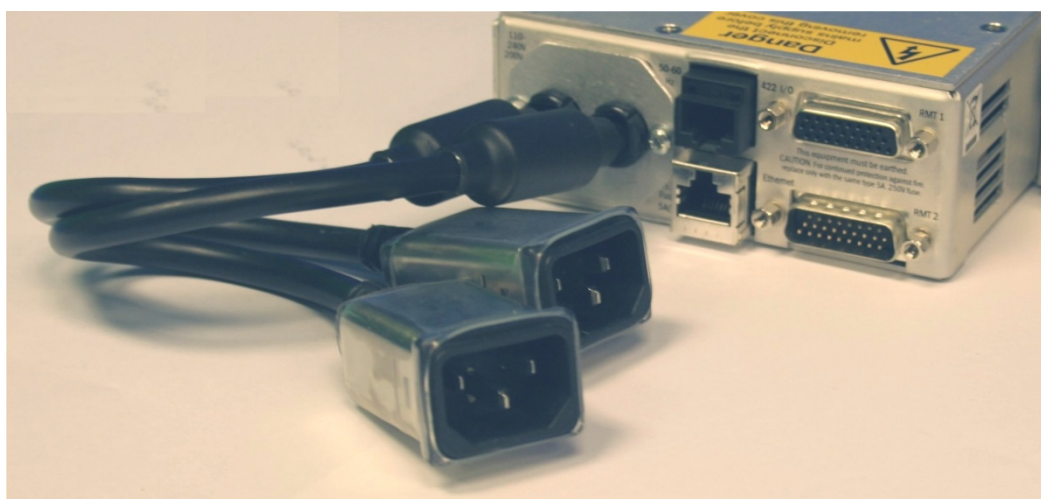
Indigo 1SE-DP/1AE-DP rear connectors
