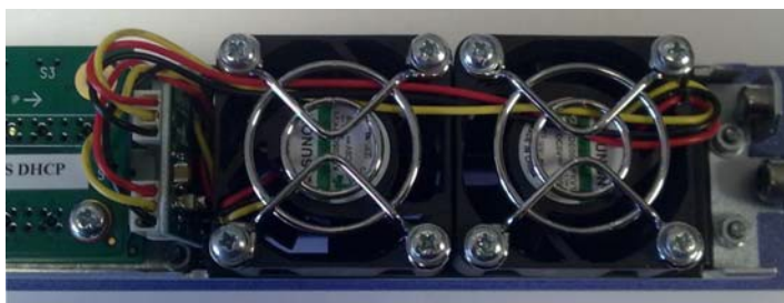
Front panel dual fans showing three-pin connectors and finger guards
