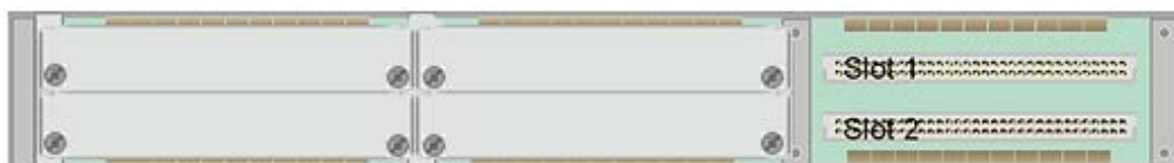
The Indigo 1SE frame rear view with EMC covers removed for slots 1 and 2
