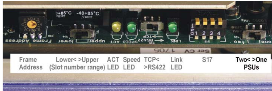
Front panel hardware settings – PSU configuration
