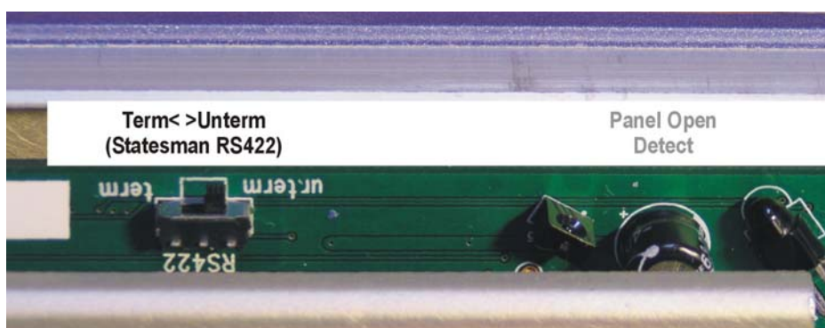
Front panel hardware settings – RS422 term/unterm switch
