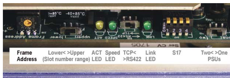
Indigo active/remote/Statesman panel hardware settings – Frame address
