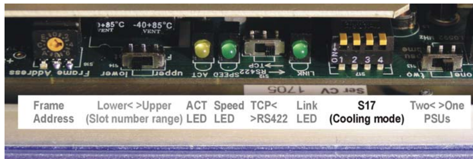
Indigo 2-48V front panel hardware settings – cooling mode
