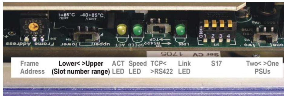
Front panel hardware settings – slot number range
