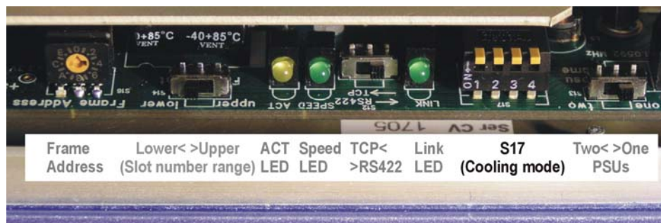
Indigo 2 front panel hardware settings – cooling mode
