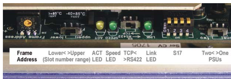
Indigo active/remote/Statesman panel hardware settings – Frame address
