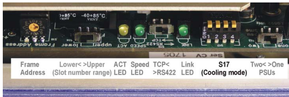
Indigo 2 front panel hardware settings – cooling mode
