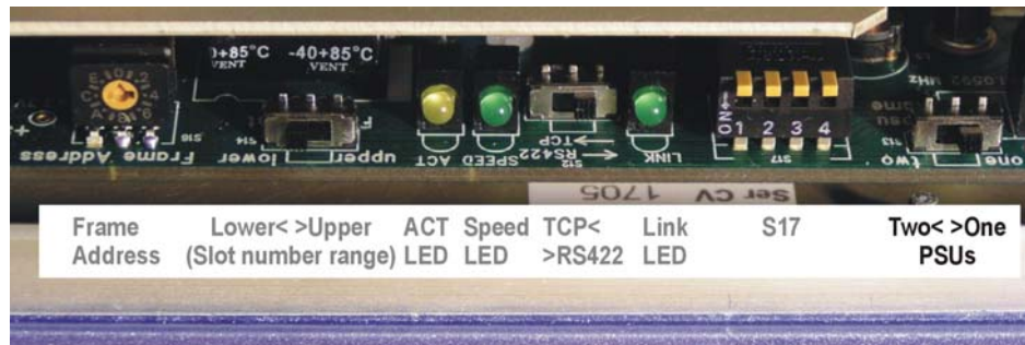
Indigo 2 front panel hardware settings – PSU configuration
