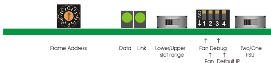
Indigo 2AE older board top-edge switches and LEDs
