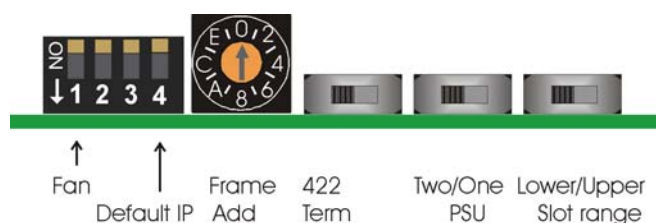
Indigo 2 front panel hardware settings – PSU configuration
