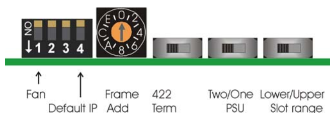
Indigo 2 CoolFlow front panel hardware settings – cooling mode
