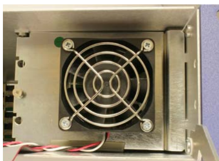
Removing the PSU fan assembly
