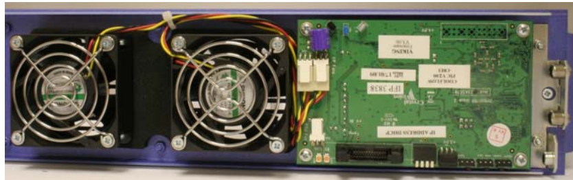
Front panel fan showing 3-pin connector and finger guard
