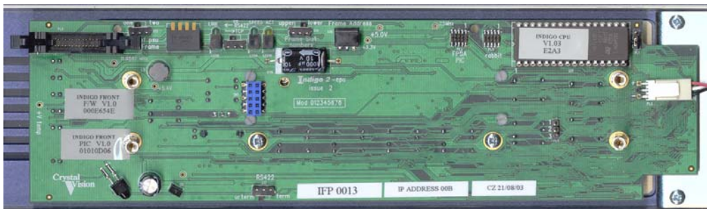
Front panel PCB with cover removed showing firmware EPROM in the top right corner
