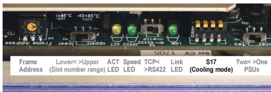
Front panel hardware settings – cooling mode (lower PCB)
