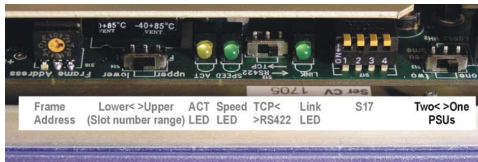
Indigo 4 front panel hardware settings – PSU configuration
