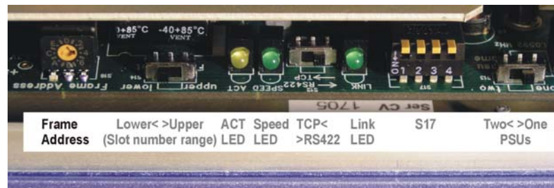
Indigo active/remote/Statesman panel hardware settings – Frame address
