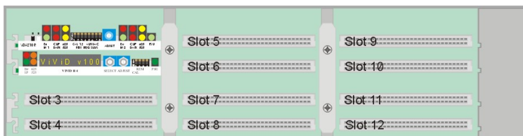
The Indigo 4 CoolFlow upper frame with two modules fitted in slots 1 and 2
