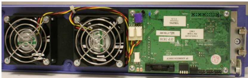
Front panel fan showing 3-pin connector and finger guard. (Indigo 2 front panel shown)
