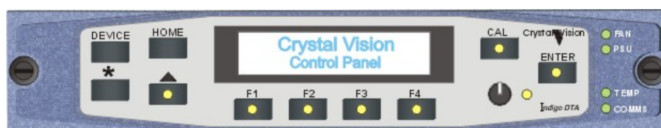
Indigo DTAE active panel controls and LEDs
