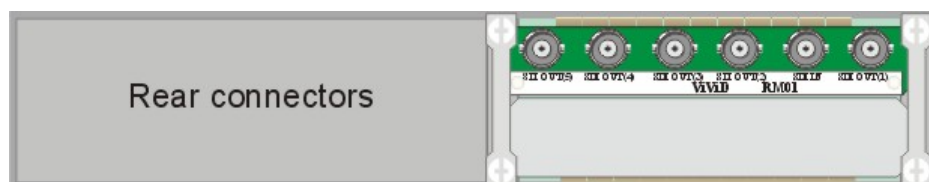
The Indigo DT with one half-size EMC cover and an RM01 connector fitted to slot 1
