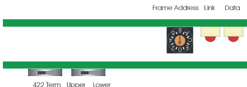
Indigo active/remote/Statesman panel hardware settings – Frame address
