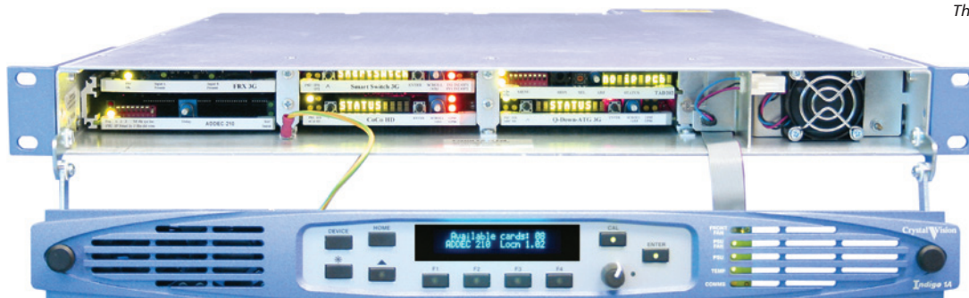
Internal view of Indigo 1AE-DP, which holds up to six boards
