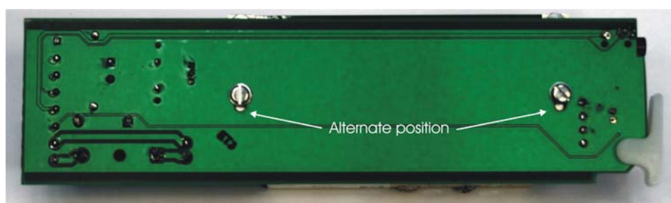
Underside of PS-55i showing alternate fixing positions
