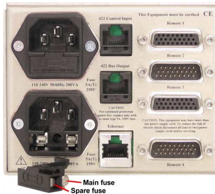
Rear connectors showing IEC mains inputs and fuse tray with main and spare fuses
