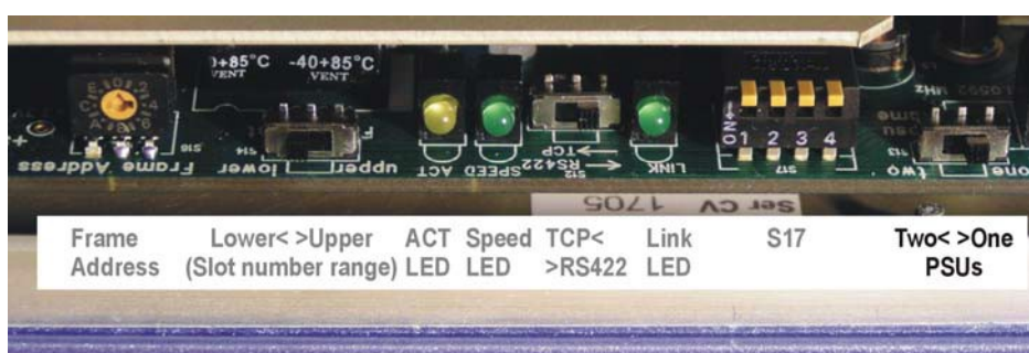
Indigo 2/2A/2S front panel hardware settings – PSU configuration
