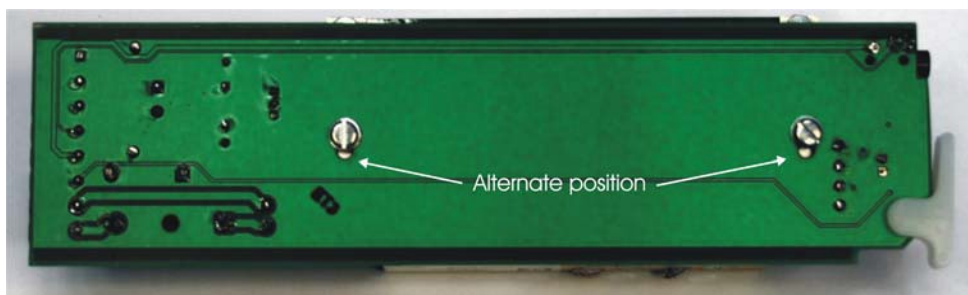
Underside of PS-80i showing alternate fixing positions
