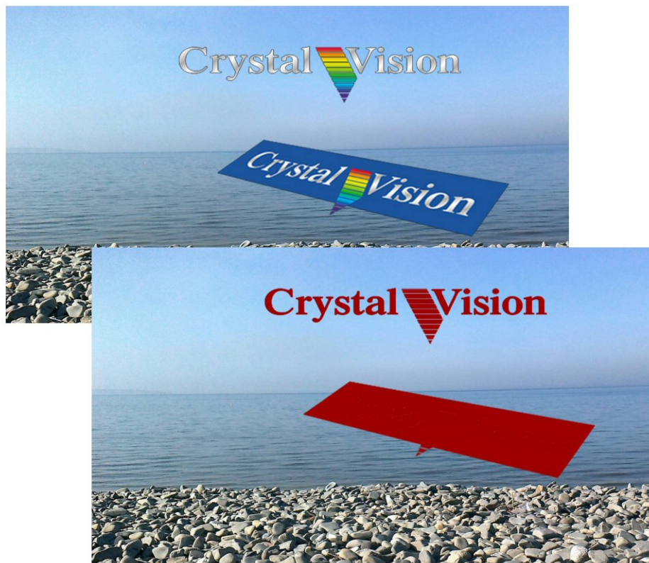
Result of Self Keying using FG Video and Matte as the FG Source
