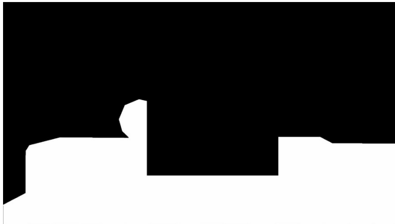
Key Output showing FG mask rectangle overriding External Key
