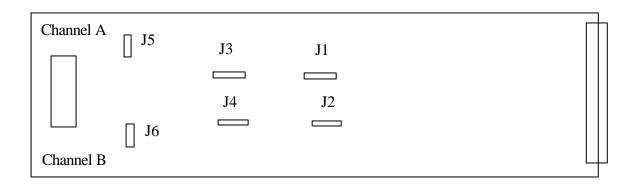
The position of the link on J5 for channel A and J6 for channel B selects either automatic or manual choice of 525 or 625 line operation.
