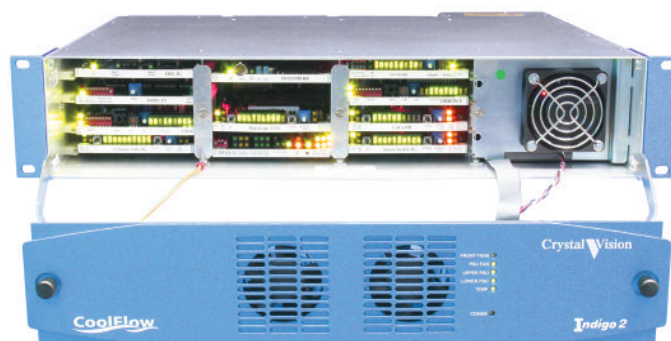
Internal view of Indigo 2, which holds up to 12 boards
