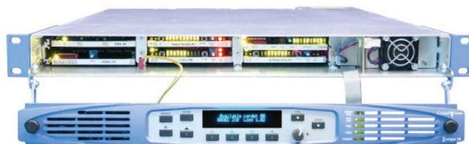
The Indigo 1AE active panel can be easily operated in the open position, thanks to the substantial hinge
