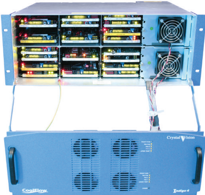
Internal view of Indigo 4, which holds up to 24 boards
