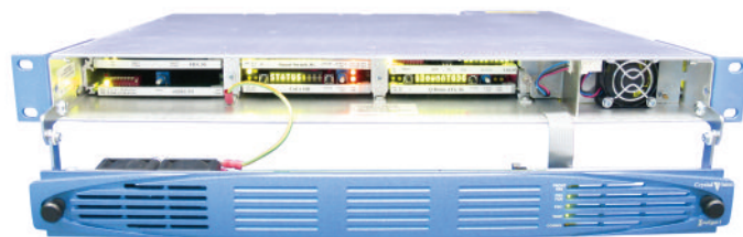
Internal view of Indigo 1, which holds up to six boards
