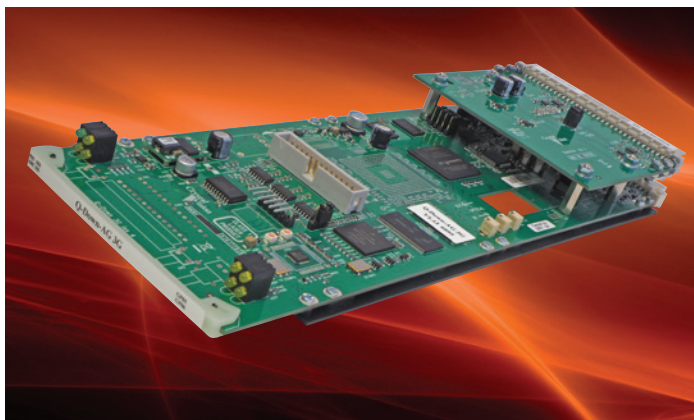
Get up to eight input loop-throughs by fitting a DA6 top board
