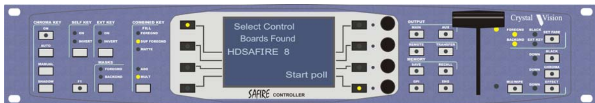
The Safire Controller Panel - one panel controls up to 7 Safire, Safire SD2, Safire HD 2, LKEY211 or LKEY HD keyers
