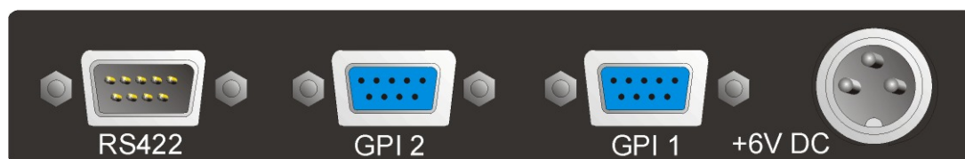
Safire Controller panel connectors
