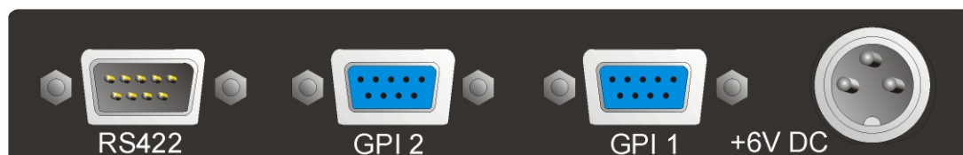
Safire Controller panel connectors
