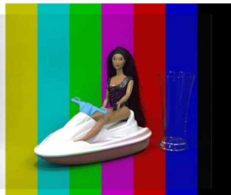
Min Clip and Max Clip misadjusted
