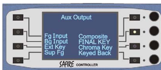
Aux output assignment – final (combined) key selected
