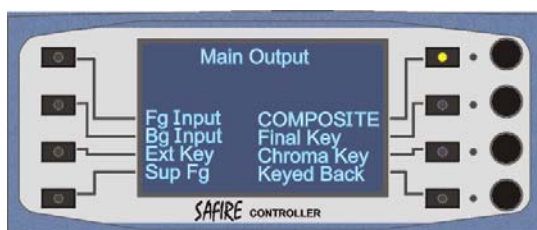
Main output assignment – composite output selected
