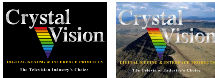
Self key over background using linear keyer
