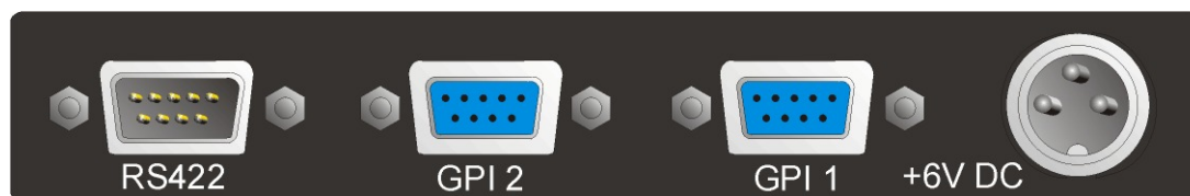
Safire Controller panel connectors
