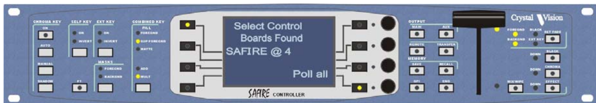
The Safire Controller Panel - one panel controls up to 15 linear chroma keyers
