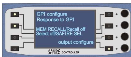
Configure GPI response for selected Safire
