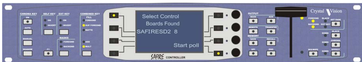
The Safire Controller Panel - one panel controls up to 7 Safire or LKEY HD keyers
