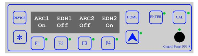
If F1 is pressed then aspect ratio conversion for Channel 1 can be turned on or off (bypass mode).
