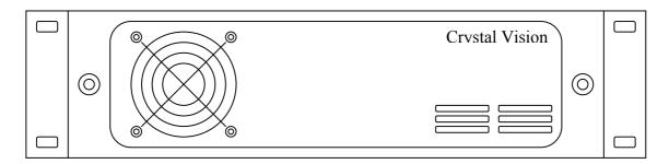
The 2U FR2AV frame will house up to 12 modules and dual power supplies. A hinged front panel gives access to the PSU and all modules. The universal frame wiring system allows any of the interface range of modules to be fitted in any position with the use of removable rear modules. All modules can be plugged in and removed while the frame is powered without damage.
