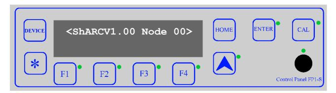
This message shows that an ShARC102 or ShARC204 has been selected with the version of software on the module as V1.00 and that node 0 is being used to address it. Depending on the software version and the node address used the output may differ from that shown above.
