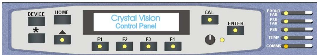
If the control panel firmware has been updated for Statesman control, Statesman mode will be entered and the message, 'Press CAL to Exit' will be displayed and the CAL LED will light.
