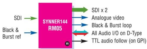
The four slot RM05 fits in the 2U and 4U frames only and can be used with either analogue audio or 110Ohm AES. It should be used for applications requiring composite video monitoring and a large number of boards in a frame.
