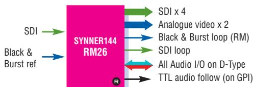
The two slot RM26 can be used with either analogue audio or 110Ohm AES. It fits less boards in a frame than the RM04 and RM05, but gives composite video monitoring and both Black and Burst and SDI loop-throughs. It can be used for applications with no piggyback, an input piggyback or an output piggyback.
