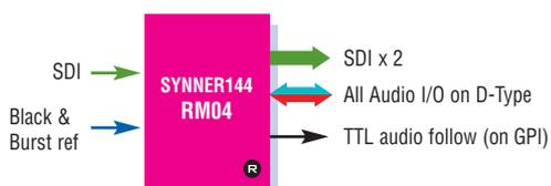
The single slot RM04 allows the maximum number of boards in a frame and can be used with either analogue audio or 110Ohm AES. It is the favourite rear module for input/output piggyback configurations where monitoring is not a requirement.
