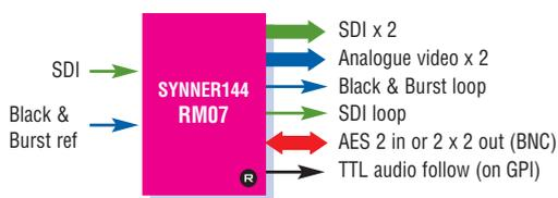
The two slot RM07 should be used for 75Ohm AES applications.
