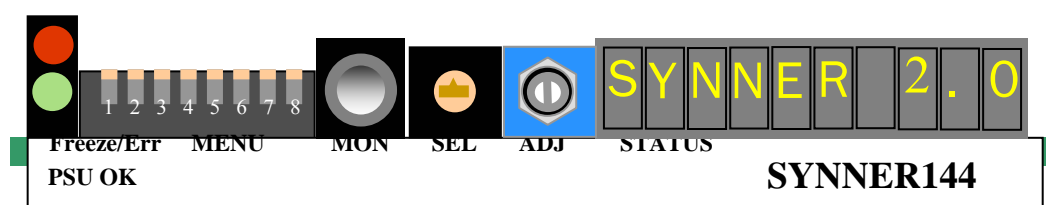
SYNNER144 front view showing controls and LEDs
