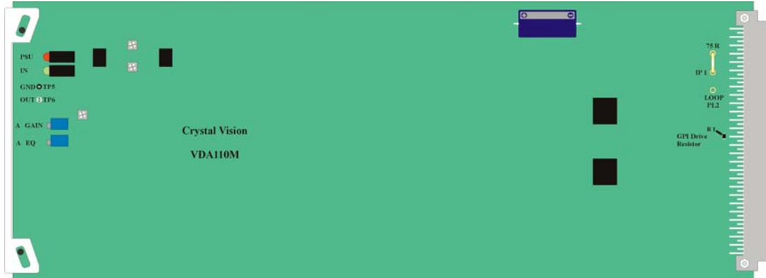
VDA110M showing termination jumper and GPI drive resistor
