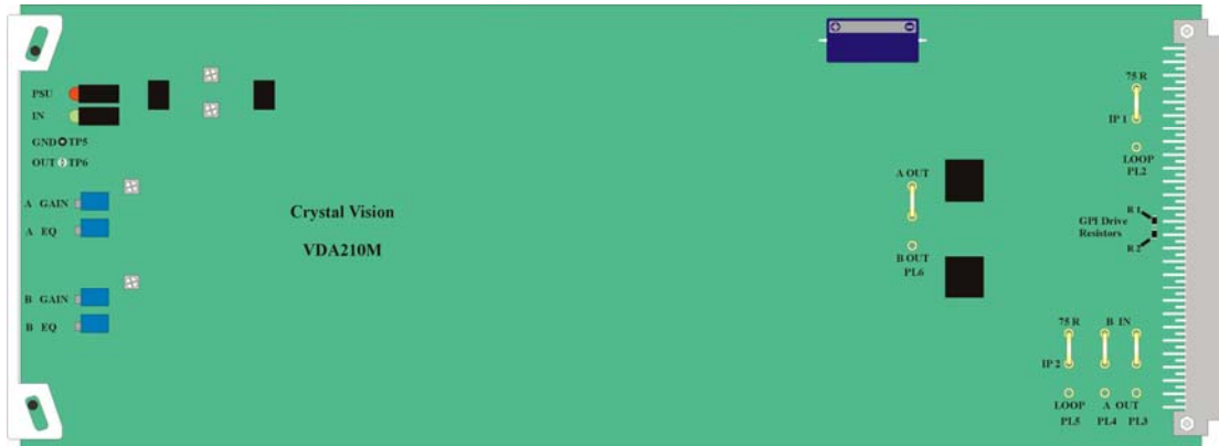
VDA210M showing configuration jumpers and GPI drive resistors
