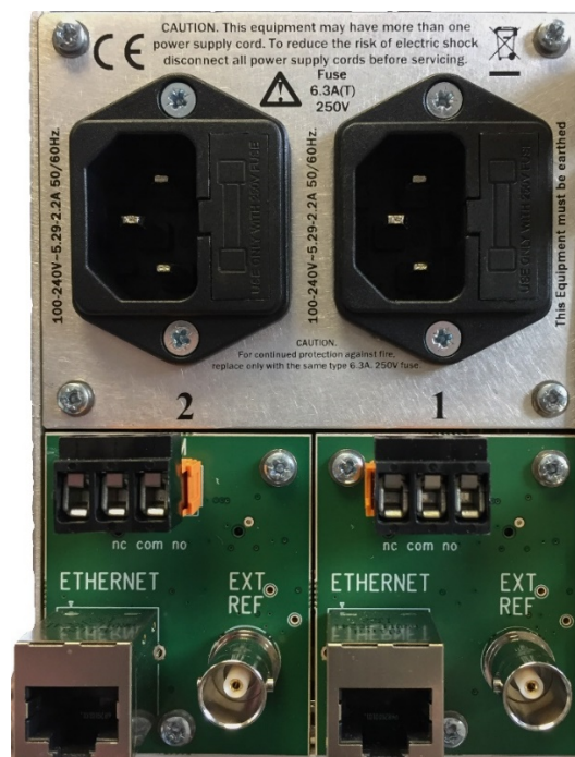
Rear view showing mains supply, alarm, Ethernet and reference connectors
