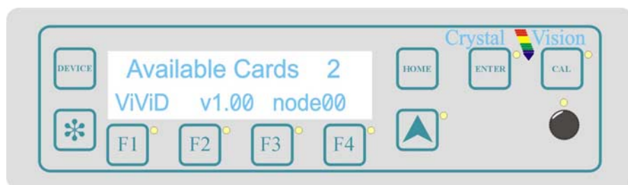
Control panel showing available cards
