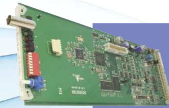
VDA110R HD: Single channel with remote control
